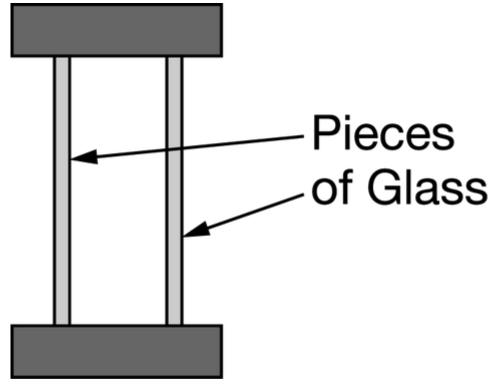
A student wants to conduct an experiment to determine the rate at which windows transfer energy to the outside air in the winter. The student investigates windows that are made from two parallel pieces of glass with a space in between, as shown in the figure. The student decides to investigate how the spacing between the pieces of glass affects the transfer of energy. Which additional criteria should the student use when selecting windows for the experiment? Select two answers.
