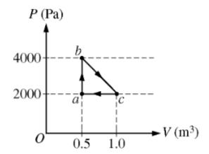
A sample of an ideal gas is taken through the cycle abca, as shown in the PV diagram above.
