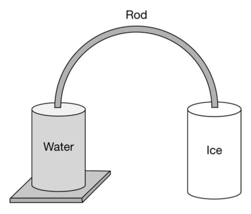
Students design an experiment with a curved, insulated rod of an unknown thermally conducting material, as shown in the figure. The rod is 1 m long and 2 cm in diameter. One end of the rod is touching the surface of water kept at 350K by a hot plate, and the other end is just touching the surface of a well-insulated block of ice.
