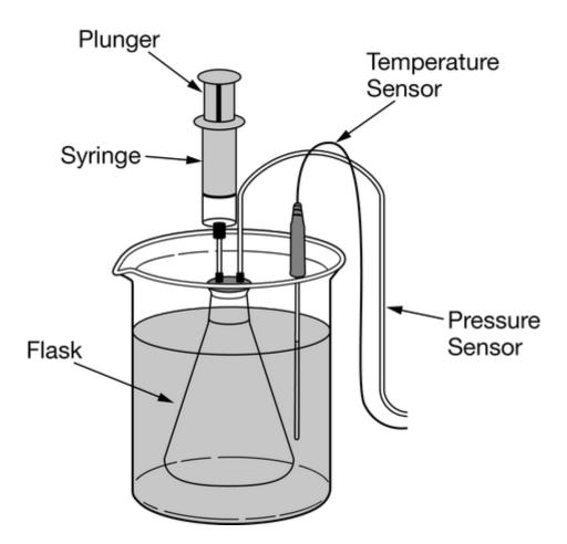
Students perform an experiment to determine the relationship between the pressure and temperature of an ideal gas. They have a flask with a stopper through which a syringe and a pressure sensor are
