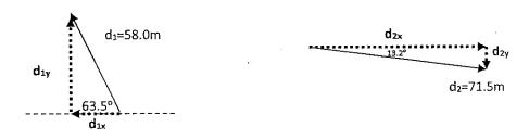
This creates two right triangles! This is because BY DEFINITION the components of a vector are always perpendicular to each other. That's good because we already know how to solve right angled triangles!
